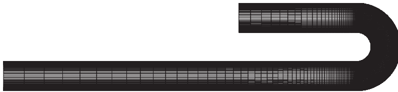
Figure 14. Computational grid for U-duct flow.
